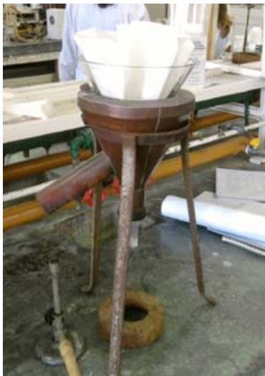
SM 12.4.1.3: Copper funnel (previously heated by flame) for hot filtration
