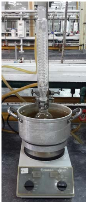
SM 12.4.1.1: Reflux apparatus for 4-nitrotoluene-2-sulfonamide
